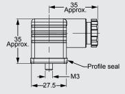
Male electrical connector 3p+PE EN 175301-803 (DIN 43650)
